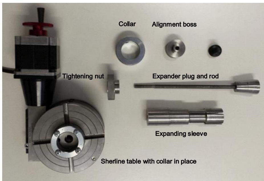
The gripping action inside the spindle is not unlike the concept of the Myford produced hand winding handle.
