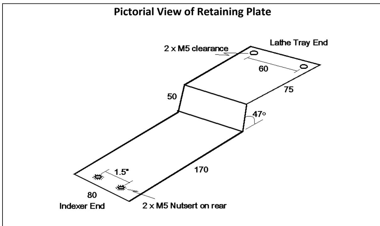
I bent a piece of 2mm x 80mm wide x 295mm long aluminium sheet with an offset bend as per the drawing above.
