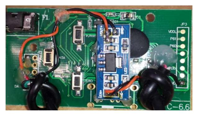
Once the mounting of the board is completed and the connections made, repeat the functionality check before connecting to the digital height gauge.
