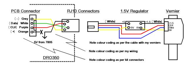
Apologies for the mixed colour codes which confuses. As drawn the wiring follows through as seen with top view of the PCB connector, bottom view of the RJ10 socket, mating orientation of the RJ10 plug and top view of the PCB regulator and the Vernier scale.
