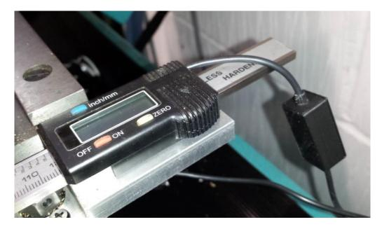
So far so good. I now had a 1.5V regulator connected close to the scale connections which if I ran from a 5V external power supply gave me stable readings on the DRO350.
