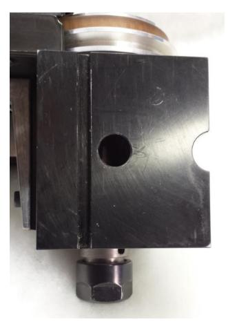
This write up details the geometry of an adapter block to allow mounting the motor on the Myford vertical slide.
