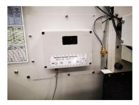
The finished boxed assembly is mounted on the ATC blanking panel on the Tormach.
