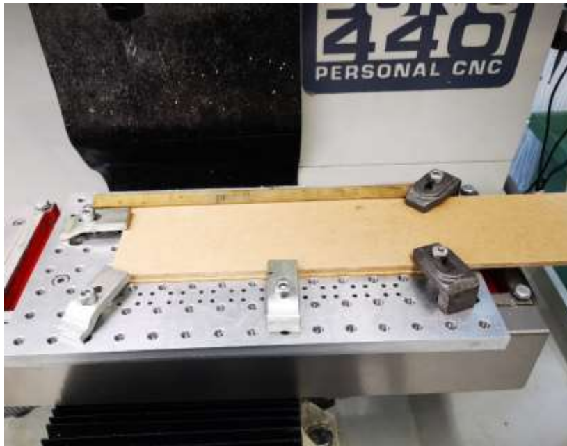
The stock and sacrificial board clamped in place against the rear Y reference brass bar
