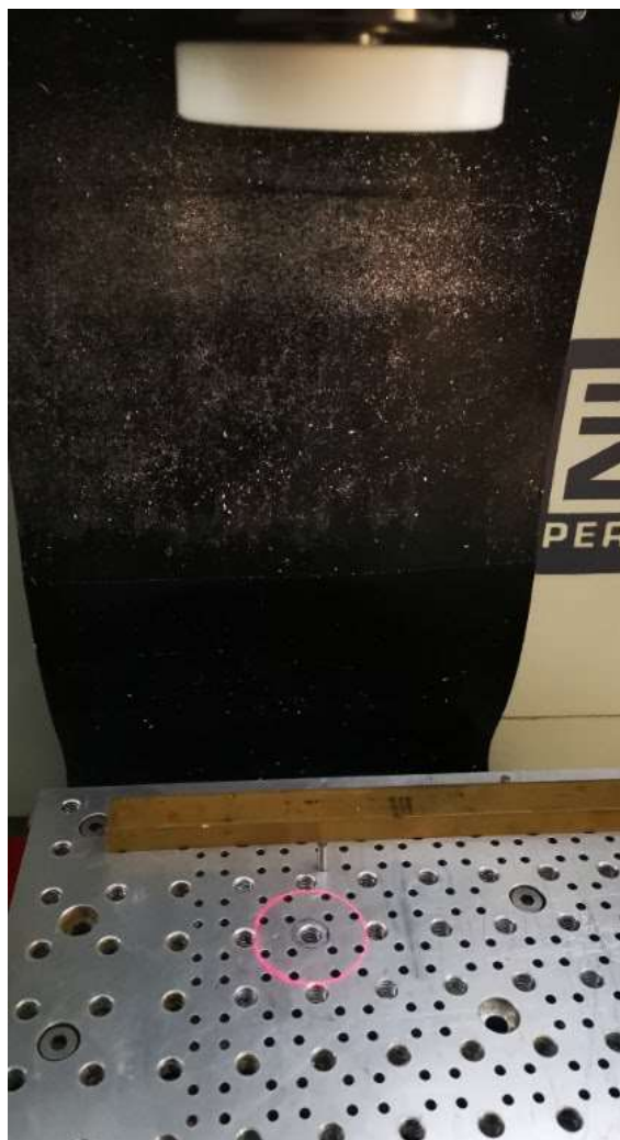
Laser Centring Tool in action showing the 'aiming' red circle and the tooling pin
