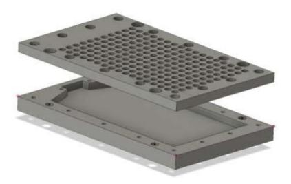
My tooling pins have a 6.8mm shank to fit into the vacuum plate matrix holes with 4mm protruding top section that engage with the MDF. Despite what you might think, MDF is very transparent to air circulation. The vacuum will therefore suck the PCB material down onto the vacuum table through the MDF.
