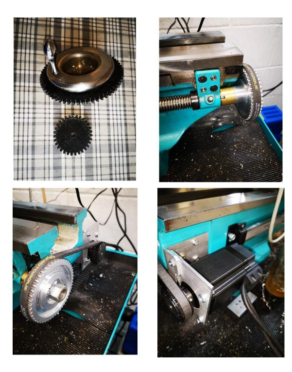
You can see the brass spacer boss and the 4mm cross drive slot.
