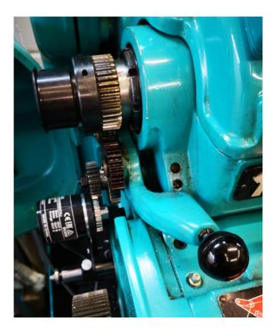
The ELS reverse facility action accuracy depends on the belt coupling from the stepper to the leadscrew. On inspection my belt was a little slack and the gear on the stepper is not running perfectly true. I need to remedy these issues and retry this method.
