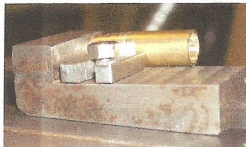
Photograph 9: Turned nozzle blank clamped in the milling jig (step 5).
