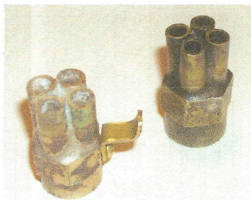
Photograph 13: One used, one new. Note thicknesses of metal showing on nozzle ends.
