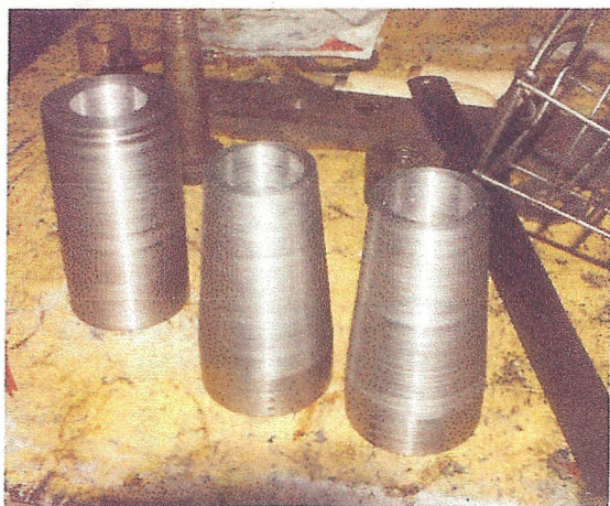
Left - Photograph 5: Lempor nozzles in process of being machined. Note taper is longer than on the miniature set.
