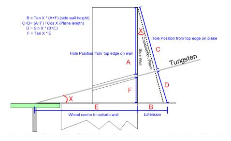
A construction plane is created at the grinding angle from the top edge of the block. This correctly aligns the grinding holes. The construction plane allows the extension B to be calculated knowing the height of the block (A+F) above the top surface of the grinding wheel. This is simple to construct in Fusion using the top edge of the block as the 'hinge' point of the plane.
