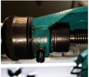
Sadly, the same protection cannot be afforded to the newly fitted top slide bearing but this area is much further away from any cutting activity so it is less exposed to debris. Clearly this is a situation to be monitored and a potential additional maintenance activity to bear in mind.
