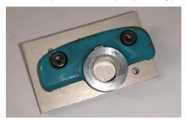
The combination of the boss skim and the collar skim delivers sufficient width gain to allow the six component parts of the thrust bearings to be accommodated while leaving the grub screw face fully able to engage with the lead screw thread.
