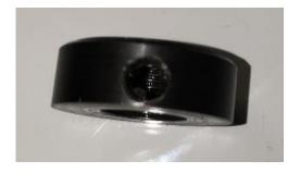
(Clearly reducing the collar raises a chicken and egg situation. You need the lathe to reduce the collar but the collar forms part of the lathe that you want to use. Either you need a second lathe or make the skim in a milling machine or you make a new collar completely which means you need to be able to cut a 26TPI thread. My small Cowells ME lathe stepped up to the challenge).
