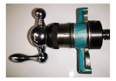
Having removed the end casting to skim it, it is important to not tighten the two locating screws down until the lead screw has been engaged with the slide and fully wound in to bring the slide up to the end of its travel.
