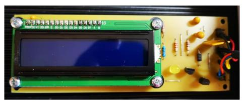
The PCB shown has an inline electronic fuse fitted and the AC inlet to the box is fused.
