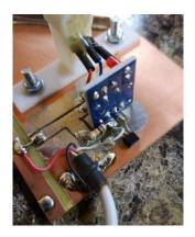
Note that the detector diode orientation and pin connections are critical otherwise damage to the device will result. If you look at the front of the body where the nodule is, the OV connection goes to the large metal electrode inside the transparent body.
