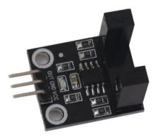
An alternative to a laser diode and detector is to us an optical coupler type device with has a light emitting diode and detector built into a single body with slot between the two. Anything passing through the slot will break the beam and cause the output to switch. Mumford supply this style of detector as standard but there are various physical presentations of these.
