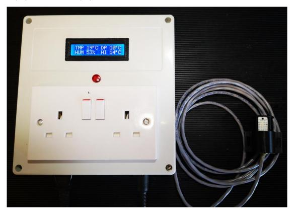
After breadboarding the design, I committed it to a printed circuit board using the Fusion 360 Electrical module. Fusion produces Gerber files which I transformed to GCode using FlatCAM. The GCode was used to mill the printed circuit board on my Tormach PCNC440 CNC milling machine. I also used Fusion 360 to give me the milling codes to mill all the cut-out holes in the enclosure and the internal mounting plate.
