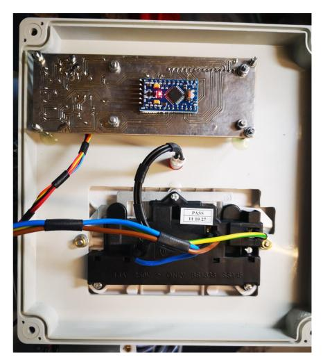
As can be seen, I like using Hellerman sleeves in my cable forms. This is far from an ideal production method as it is slow and tedious. It does allow you to be flexible in the cable routing and does allow mistakes to be easily rectified. You do need Hellerman pliers for this technique and I use DC4 silicon grease as the lubricant.
