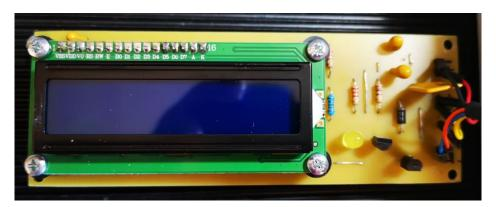
Not wanting to have additional holes in the box front panel, I used Araldite to glue four countersink screws to the inside face of the front panel and mounted the display off these.
