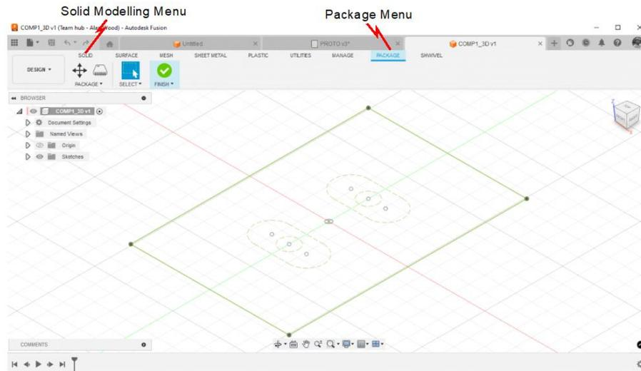
Go to the Solid Modelling Menu to enter the modelling module. The screen will redraw but now with the familiar 3D modelling icons showing across the top line. The faint image of the footprint COMP\_FP will remain centred on X0,Y0,Z0.
