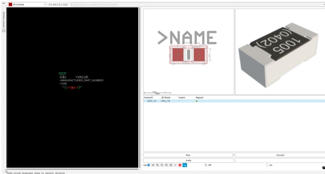
Connect the schematic symbol to the footprint.
