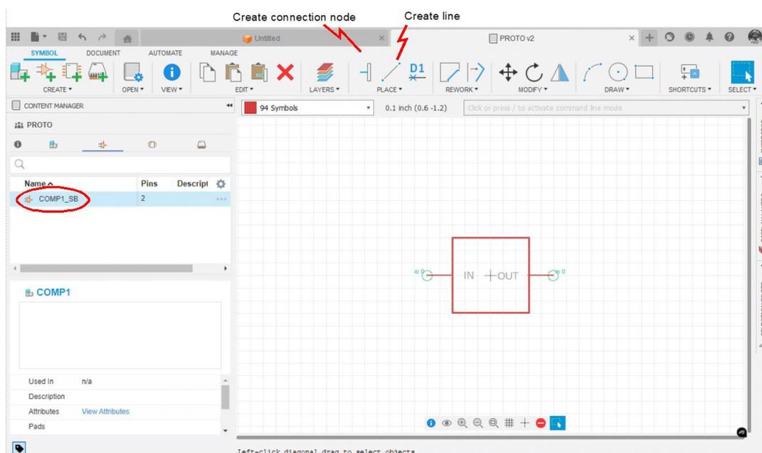
**Warning :** When creating symbols, do not vary the creation grid from the default values (0.1"/12.7mm) or your circuit connections will not mesh with the node handles on the symbol.
