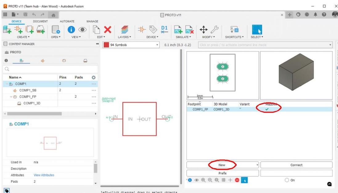
You can expand the view of what the component file contains using the indenting arrows in the left hand box. You can right click and Rename any of these should you wish.
