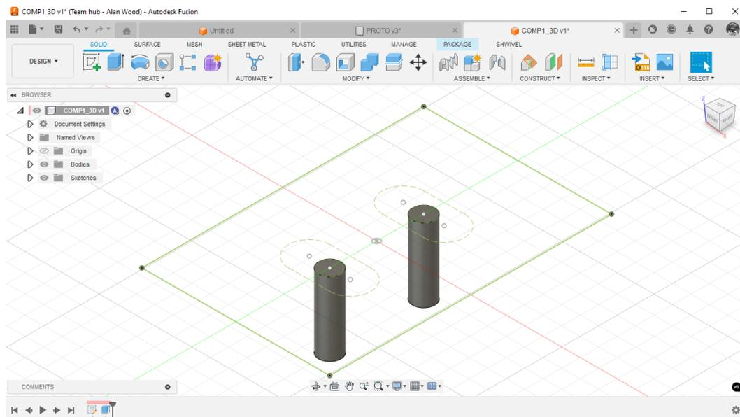
Next sketch a centred box on X0 Y0. This should closely match any dimensional information you have from the manufacturer of the component. As our part is fictional just make it similar to the existing sketch of the silkscreen outline. Extrude upwards for +5mm. Make sure this is a Join operation so the pins and box are one item. Save this which will be a User Save.
