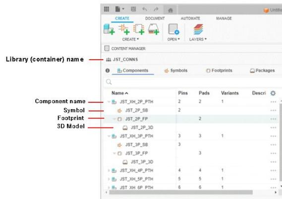
If I needed to, I can now add a new version of a JST connector to this library. This will involve creating a new symbol, new footprint and a new 3D model. To keep my sanity, I suffix each part of the component constituents with SB, FP and 3D but you can use whatever method of naming that helps you get the desired result. The names are not important, just how the named parts ultimately mesh together. If you want to change any of these visible names then a right click offers a Rename function.
