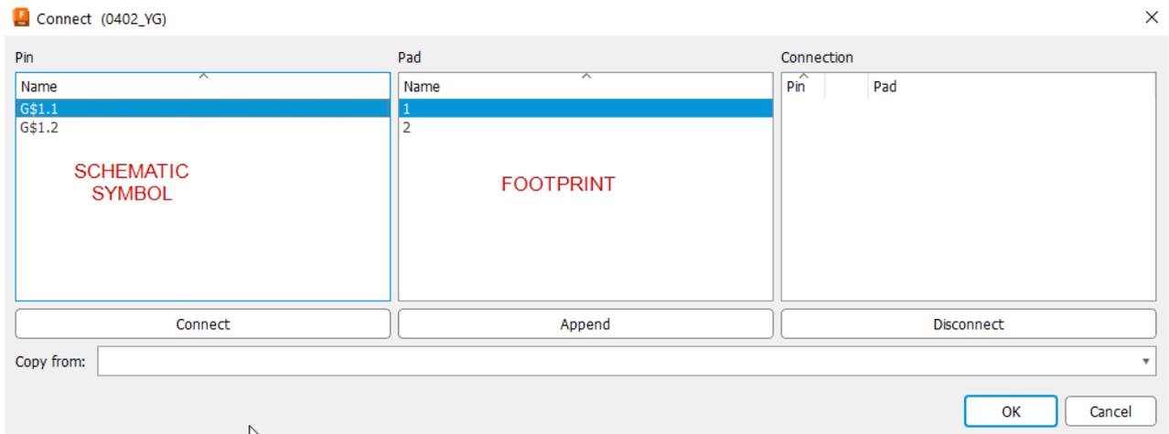
Connect schematic symbol pin 1 (G\$1.1) to footprint pin 1.
