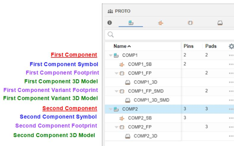
Just as a cross check here is the view when selecting a component from the PROTO library with the drop arrows revealing the two variants of COMP1.
