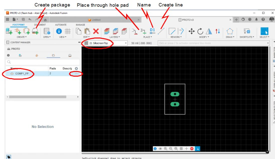
Notice how with each step taken so far, the blue highlighted name in the left hand box only shows the name of the part currently being created (i.e. there is no inter part relationship apparent or tree structure as yet).
