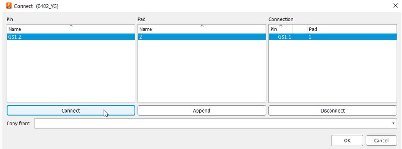
Connect schematic symbol pin 2 (G\$1.2) to footprint pin 2.
