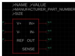
Figure 1: Schematic Symbol
