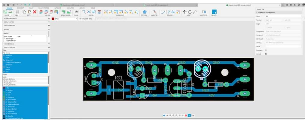
Note that with all highlighted blue in Types and Layers this gives full access to all aspects and you can then select one particular line to focus by type. Use Click at the top and bottom with Shift to reselect all or in Layers use the Default Presets. For multiple selections hold CTRL and Click as wanted.
