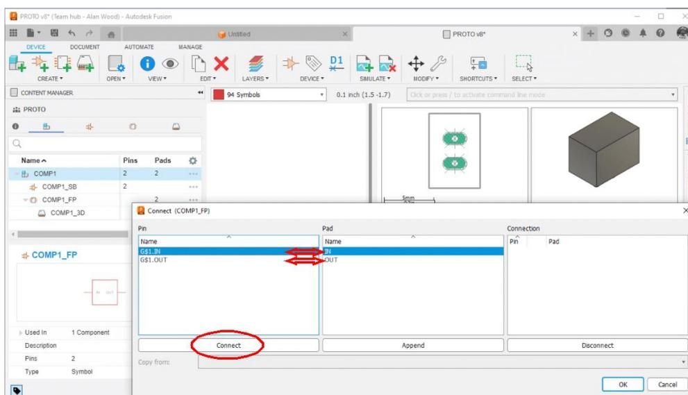
This is a simple process of linking pin names to pad names. Go down the list in the Pin window and click on the associated Pad name and then click Connect. The pairings will then move across into the Connection window. The example that has been created for COMP1 will only have IN and OUT to be linked. Once this is done press OK. A tick will appear in the Mapped column as shown below.
