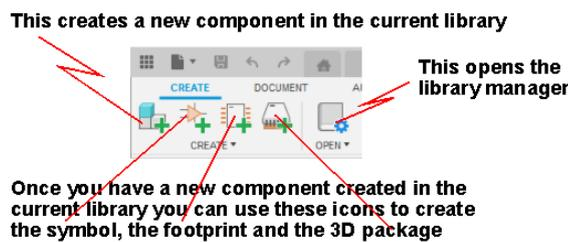
The new component is created using the above icons in sequence. The icons are only used for creating the component and its constituent parts NOT creating the library which is done via the File menu. This is an important differentiation. In this example we do not need to create a new library container file as we are adding to an existing library and working within it.
