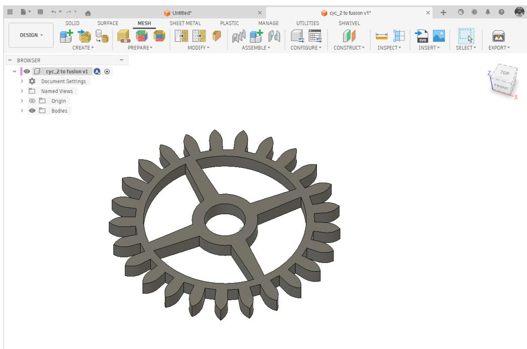
This completes the STL wheel importation and solid conversion using the licenced version of Fusion. The solid model is fully editable to add or modify features. If you need to create a CNC program from the solid model then go to the Manufacturing work area and create your setup and toolpaths as you normally would.
