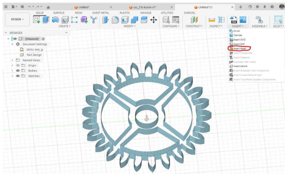
Zoom into the skeleton wheel and notice that the shape is made up of triangles (sometimes called facets). This is how 3D models are constructed. Any shape can be broken down into triangles. The first step is to 'repair' the STL model to have infill. Go to the Mesh tab and click on the Repair icon as shown below. This will bring up the sub menu as shown.
