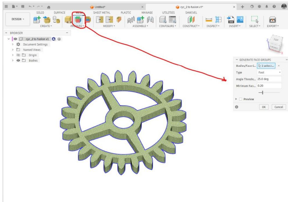
The transformed image will show colour in some of the wheel areas. The mesh is now ready to Convert to Solid. This function is found under the Modify tab. Set the parameters as shown and then OK. You will almost certainly get a warning that the model has in excess of 10,000 triangles and could take some time to compute.
