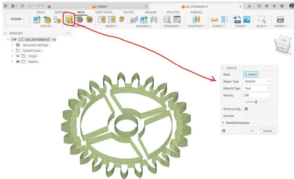
The result of the Repair will be an infilled model which has changed colour to a light blue. If you zoom in closely you will see the number of triangles has gone up dramatically.
