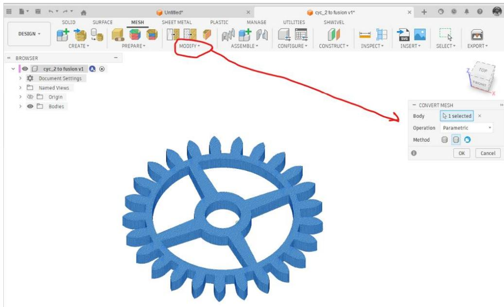
After a short while you will have a solid version of your wheel as shown below. This can be sent to a 3D printer with all the repairs already completed and with no need for the slicer to do anything other than prepare the wheel for printing.
